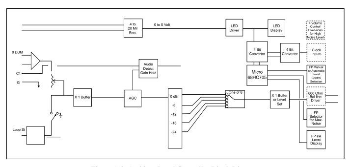
Figure 1-3. Ambient Level Controller Block Diagram
